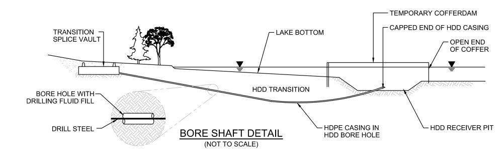
1. COFFERDAM TO BE UTILIZED WHERE NECESSARY TO STABILIZE BOTTOM SEDIMENT AT HDD TERMINUS.
